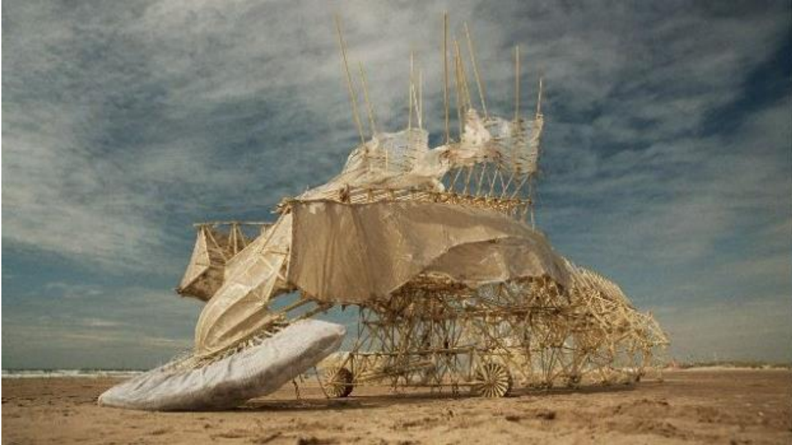
Figure 3. Strandbeest creation that will walk across a beach using only wind power
