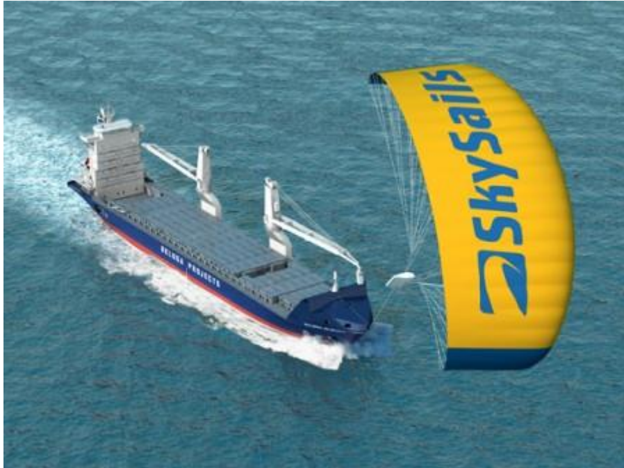
Figure 2. Skysails used for towing boats so no electricity is used
